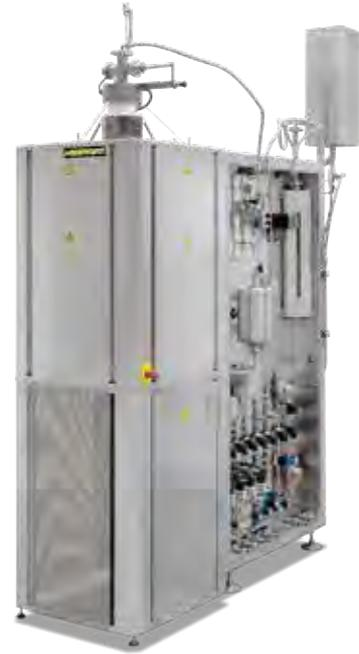
RHTV 120/600/17 H<sub>2</sub> with gas supply system 4 for flammable gases, swiveling hook for hanging the batch and safety door in front of the lower flange
