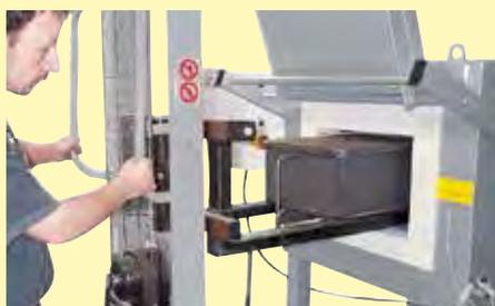
Working with protective gas boxes for a protective gas atmosphere using a charging cart
