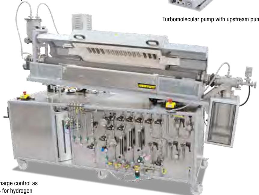
Rotary tube furnace RSRC 120/1000/11 H<sub>2</sub> with three-zone control, charge control as well as FeCrAl working tube, feeding system and gas supply system 4 for hydrogen operation
