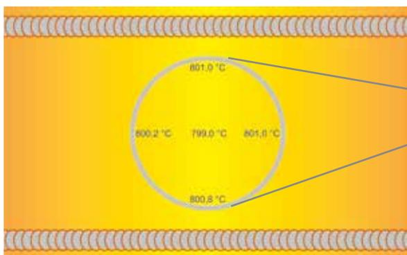
Temperature uniformity, measured in tube furnace RSH 170/750/13
