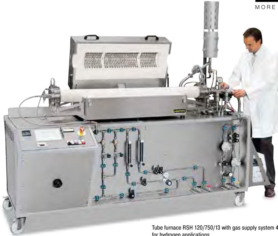
Tube furnace RSH 120/750/13 with gas supply system 4 for hydrogen applications
