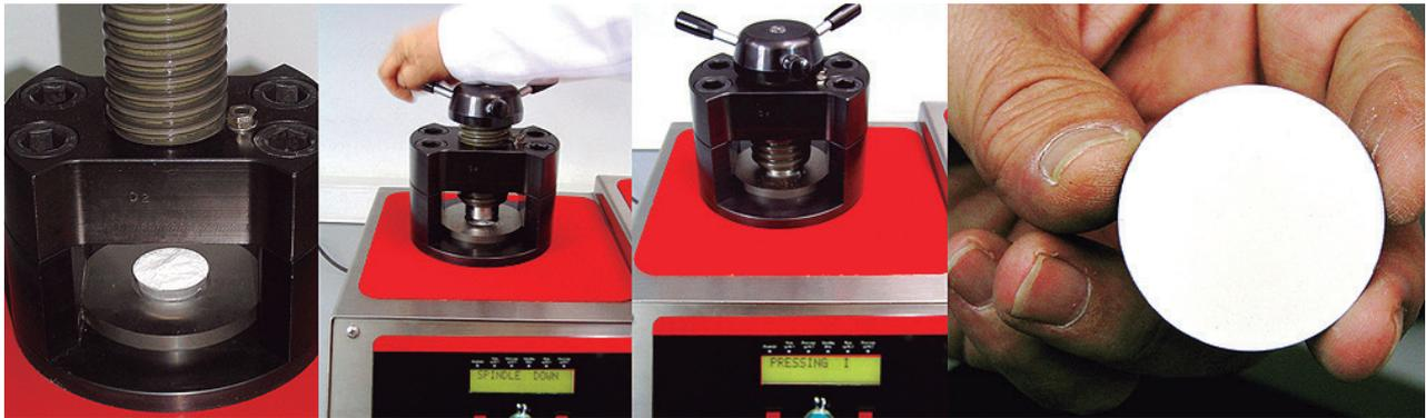
The technique consists in compressing the particles of the dust sample (by themselves or with a binder) until getting a perfectly homogeneous disk with a flat surface, mechanically robust and without cracks or dust.
