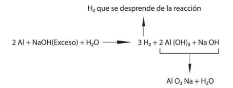
The H<sub>2</sub> released from the reaction, kept sealed under a constant volume and stable temperature conditions, will generate a pressure increase proportional to the percentage of metallic aluminium in the sample.
