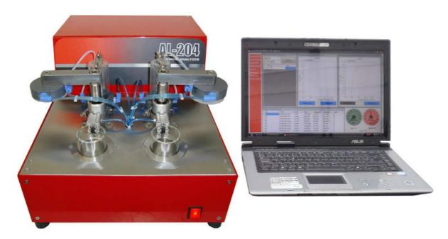
The AL 204 equipment has been specially designed for fast and accurate determination of the concentration of aluminum in metal slags. Through the analysis of gases resulting from the attack of the sample with sodium hydroxide (NaOH) can be obtained quickly - in just 10 minutes - and accurate - accuracy >99% - the percentage of aluminum content in the sample.
