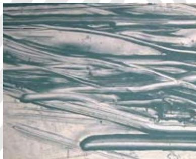
Identification of microcracks with ambulatory metallography
