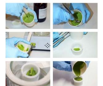
1-Mix Technovit 4002 IQ. 2-Dip in porous specimen.
