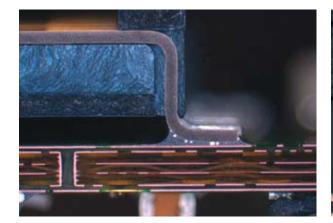
Gap-free mounting of an SMD plug from the electronics of a mobile phone in the dark field
