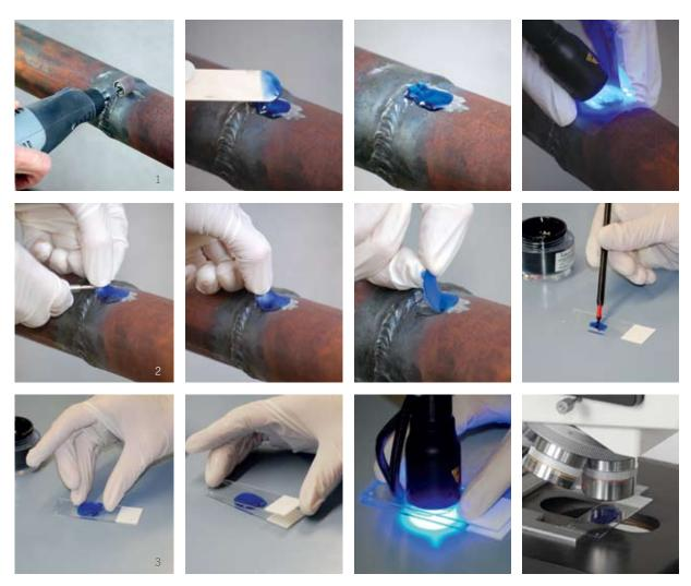
1. Grind slightly, polish, etch, apply Technovit 2220, spread thinly with a film, cover and polymerize.
