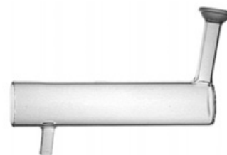
250-12 - Scott Spray Chamber, 190400-65
