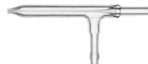
500-72 - C-Type Concentric Nebulizer, 1 lpm Ar, 30psi, 3mL/min
