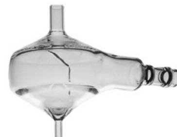
800-21 - Cyclonic Spray Chamber, 8mm Top, 4mm Drain, 20-100817-00
