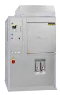
High-temperature furnace HT 160/17 with gas supply system
