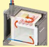
Schematic presentation of air circulation in ashing furnace L 24/11 BO
