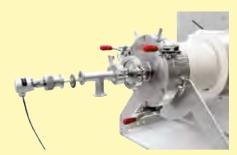
Thermocouple for charge control
