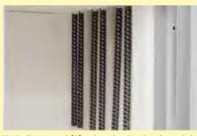
Vertically mounted SiC rods and optional perforated air inlet tubes of the debinding system in a high-temperature furnace
