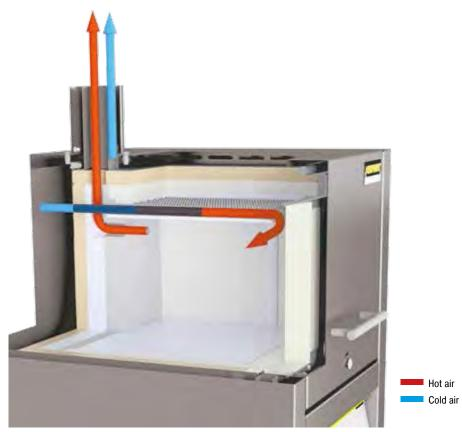
Air inlet and exhaust flow principle in ashing furnaces
