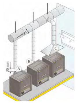
Various ways of removing the exhaust air
