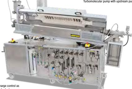
Rotary tube furnace RSRC 120/1000/11 H<sub>a</sub> with three-zone control, charge control as well as FeCrAl working tube, feeding system and gas supply system 4 for hydrogen
