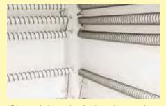
LF furnace design provides for shorter heating and cooling times
