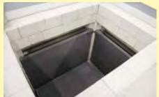
Sides and floor lined with silicon carbide tiles as protection for pit-type furnace S 73/HS
