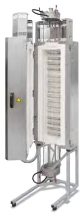
Tube furnace RSV 170/1000/11 with gas-tight quartz glass working tube and water-cooled vacuum flanges
