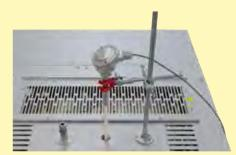
Thermocouple port in the ceiling with tripod
