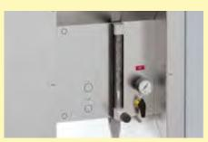
Automatic gas supply system with solenoid valve and rotameter
