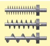
Screw-conveyors with different pitches
